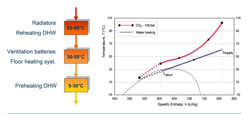
Falling return temperature in the heat distribution system increases the COP for the  $CO_2$  heat pump  $\Rightarrow$  Serial connection of heat loads at falling temp. levels
